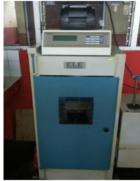
Gambar. 2 Alat uji tekan ( Compression Testing Machine ) Sumber: Data Olahan, 2023
